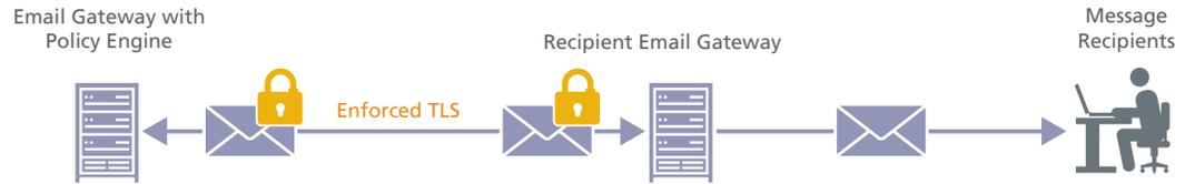
Automated gateway-to-gateway encryption protects data in motion without relying on the end-user.
