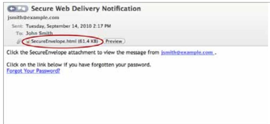
Example of a Push-based encrypted email delivery. The message includes an encrypted HTML attachment that can be opened with a browser.
